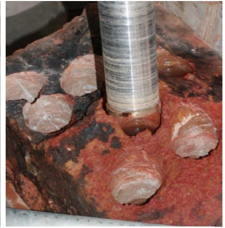
Fig. 2.3-3: Drilling Samples in the Nickel-Silicate Block
