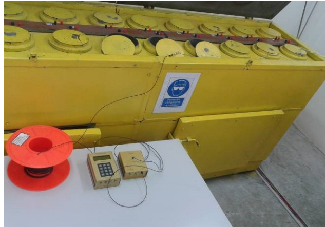
Fig.4. The measuring and command equipment for the stand for determine the precision of detonators delay
