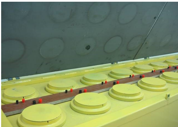
Fig.2. Stand for testing electric detonators as required by harmonized European standards
