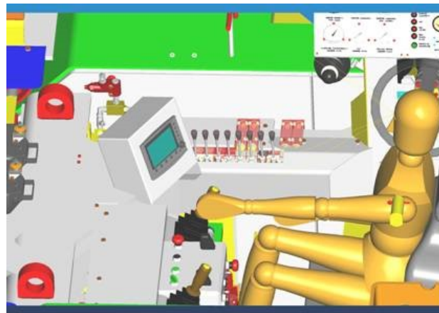
Figure 14: Result of a simulation of the operator's access to the control desk during the drilling-bolting processes in terms of ergonomics of the operator's work during operation in the mine face
