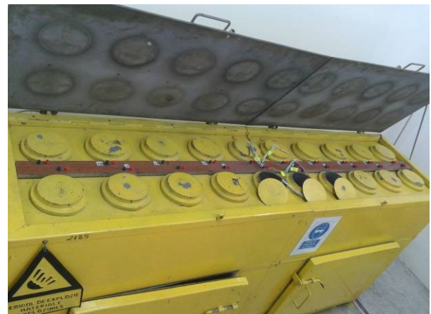
Fig. 3. Electric detonators prepared for testing
