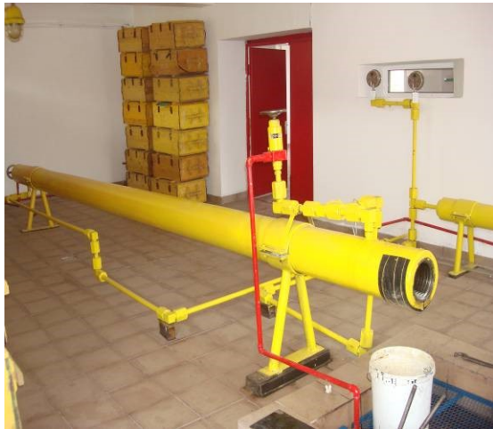
Fig.5. Stand for pressure conditioning
