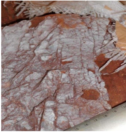
Fig. 2.3.1: Closely jointed Hematite Sample
